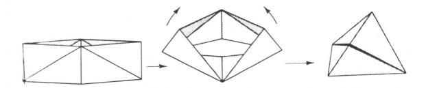
Here is a neat way of making a tetrahedron which can fold that in an instant. All that is required is a rectangular piece of card 28 cm long and 4 cm wide. Divide the long rectangle into four smaller equal rectangles and mark in the diagonals shown.
